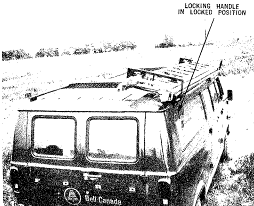
Fig. 35 — Ladder Locked in Position on Roof-Mounted Ladder Bracket
